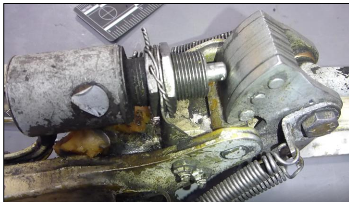
Photo No. 5: Latch at switch actuation position
