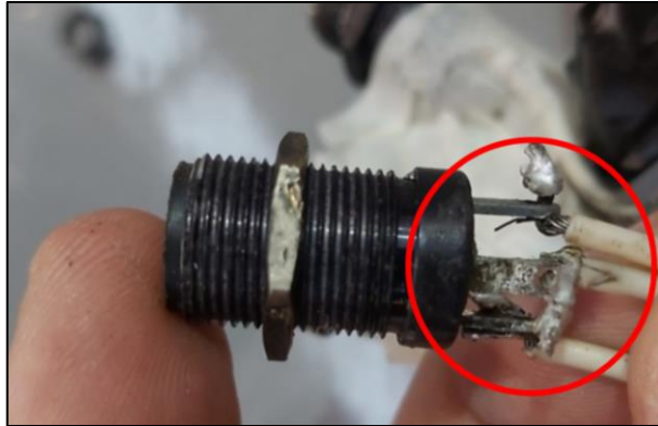
Photo No. 6: Condition of soldered joints (circled) at nose landing gear indication light fitting
